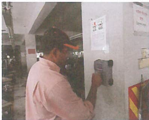
(a) Use of re-bar detector
