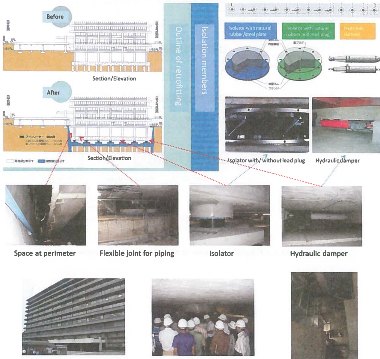
Central Government Building No.3, Isolator at the basement Expansion Joint at ground floor level (Courtesy: Ministry of Land, Transport, Infrastructure and Tourism, Japan)
